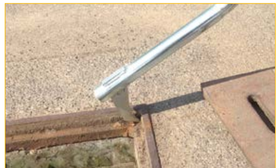
The "Nail" can also be used for cleaning the manhole frame from rusting and as a strong scourer inside the frame.
