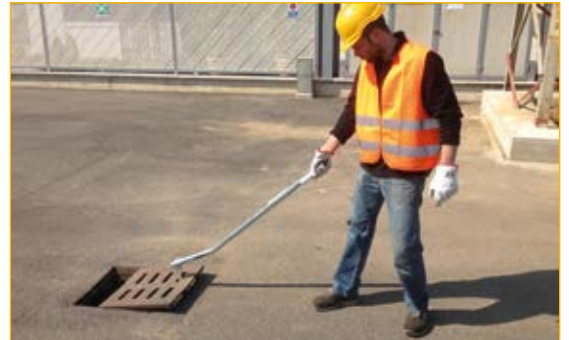
The particular angle of the lever allows an ideal ergonomics for standing operators.
